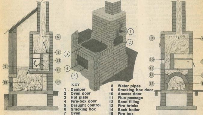
One of the most useful and innovative ideas in John Seymour's book is the "Fachongle Furnace" which is designed to yield the maximum possible benefit from the burning of wood. The furnace provides space heating for a large area, a lot of very hot water, a hot plate and oven for cooking, and a smoke chamber. The Wood is burnt in a tunnel made of fire bricks. The back is closed off and contains the back boiler for water. The front comes almost up to a hole in the house wall where there is a fire
