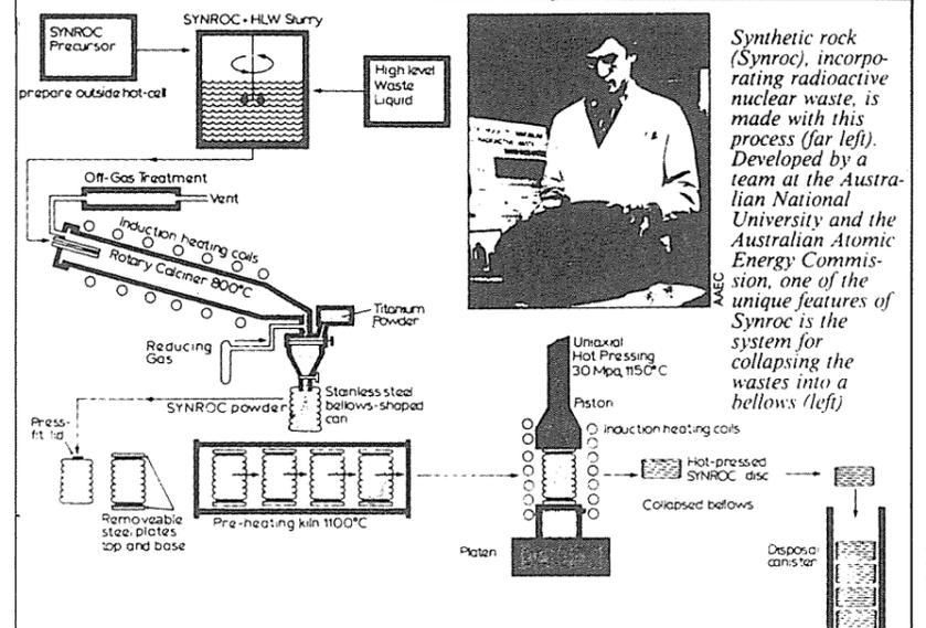
**Schematic diagram of Synroc production**
